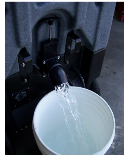
Draining the Recovery Tank
