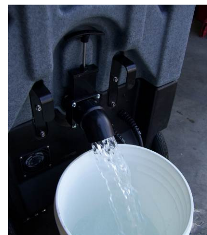
Drain water from Recovery Tank
